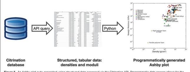
Figure 5. An Ashby plot auto-generated using structured data accessed via the Citrination API. Programmatic data access allows for the construction of key materials data visualizations, such as Ashby plots, without tens of hours of manual data entry. Note: AISI, American Iron and Steel Institute; GFRP, glass-fiber-reinforced plastic; CFRP, carbon-fiber-reinforced plastic.
